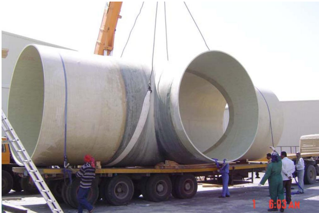
Figure 2.6: Very large FRP pipe T-connector ( www.futurepipe.com )
