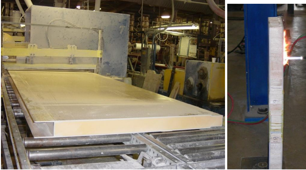
Figure 2.14: FRP application for ship decks L); successful testing of fire resistant FRP panel at 5800 degree F with acetylene torch for 5 minute at CFC-WVU. (Courtesy: CFC-WVU)
