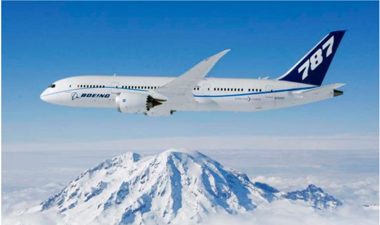
Figure 2.11: Boeing 787 Dreamliner , the world's first major commercial airliner to use composite materials for most of its construction ( www.boeing.com )
