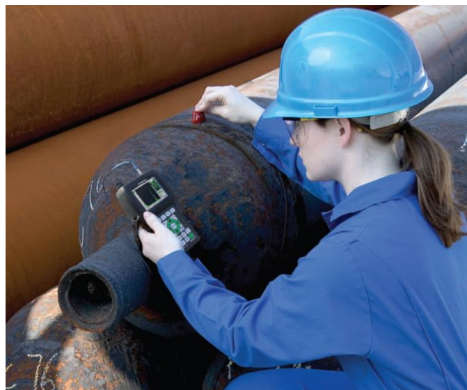
Figure 7.4: On-site ultrasonic inspection, (www.olympus-ims.com)
