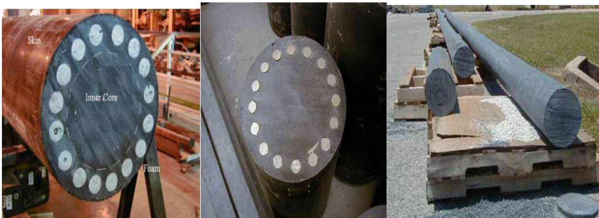
Figure 2.7: Composite marine piles from different manufacturers were tested. Shown in pictures: SEAPILE, PPI and Trimax piles, (Juran and Komornik, 2006)
