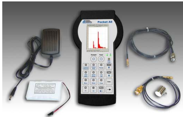
Figure 7.2: Single channel handheld AE device with sensor and accessories, ( www.envirocoustics.gr )
